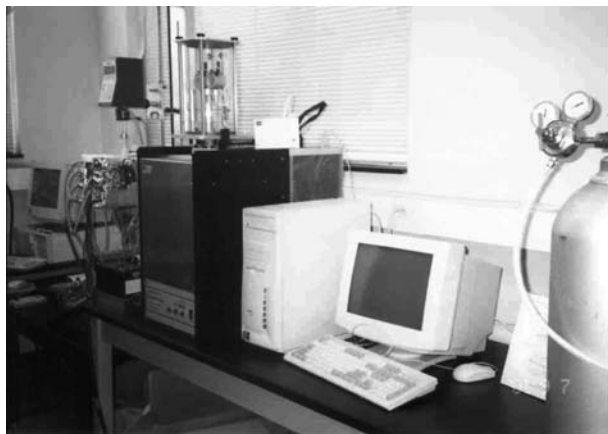
Fig. 1. Computer-controlled dual-pushrod Unitherm TM Dilatometer (Model 1161V, Anter Corp.) to measure the density and the thermal expansion of mold materials.
